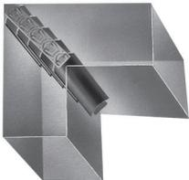
Additionally, turning vanes are designed to spread the return air more evenly across the filter so that particulates do not accumulate in one section, which can reduce the filter's performance and potential service life.
